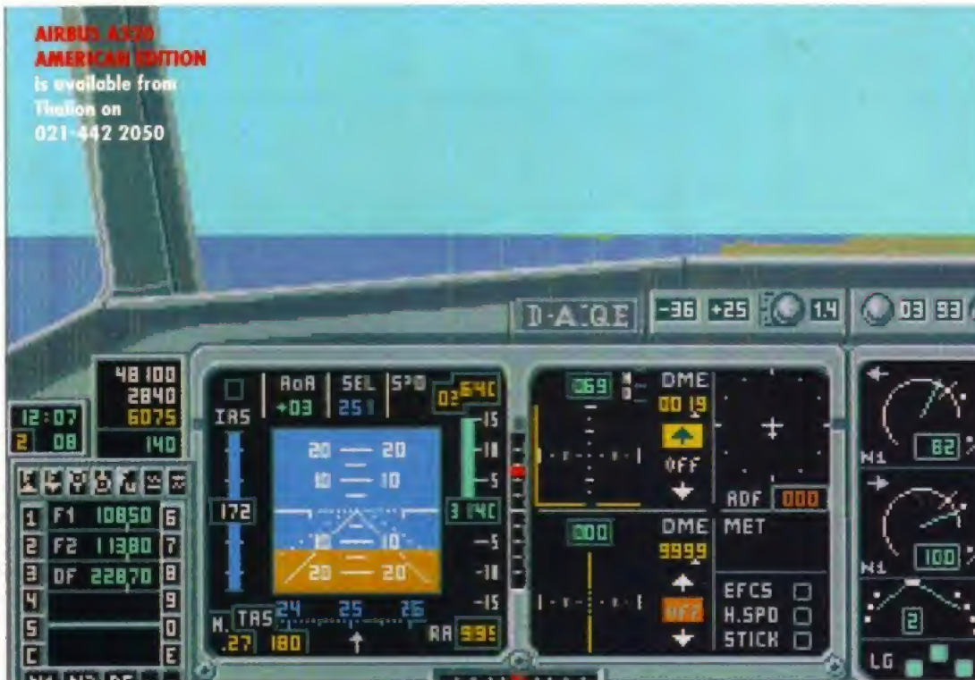
This main cockpit display is what you'll be seeing most of in A320. The numbers in blue at the bottom left (next to F1 and F2) are your start and destination points. The number next to DF is the local radio frequency.
